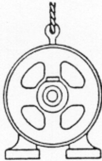
Vertical lift on eyebolt is good practice
